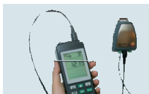
Inspection of transmitters with 4 to 20 mA interface
